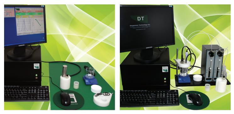
**Models DT-300** and **DT-310** have a unique **Electroacoustic sensor**, which is built as a probe (see on the right) for measuring  $\zeta$ -potential in concentrates without dilution. The same probe can be used for monitoring sedimentation kinetics.
