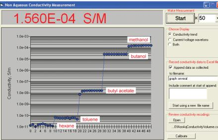
**Model DT-700** is a stand alone instrument for measuring electric conductivity of low polar (alcohols) down to completely non-polar liquids (toluene, hexane, etc) within the range of 7 orders of magnitude. This measurement can be used for studying ionic composition of such liquids, which affects many properties of the liquids, emulsions and dispersions. Consequently, this instrument is suitable for the quality control of these properties.
